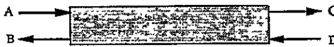
Figure 2. The input and output amplitudes from a one-dimensional disordered wire, which are related by the scattering matrix.
